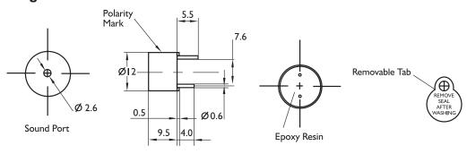
Dimensions : Millimetres Tolerance : ±0.5mm
